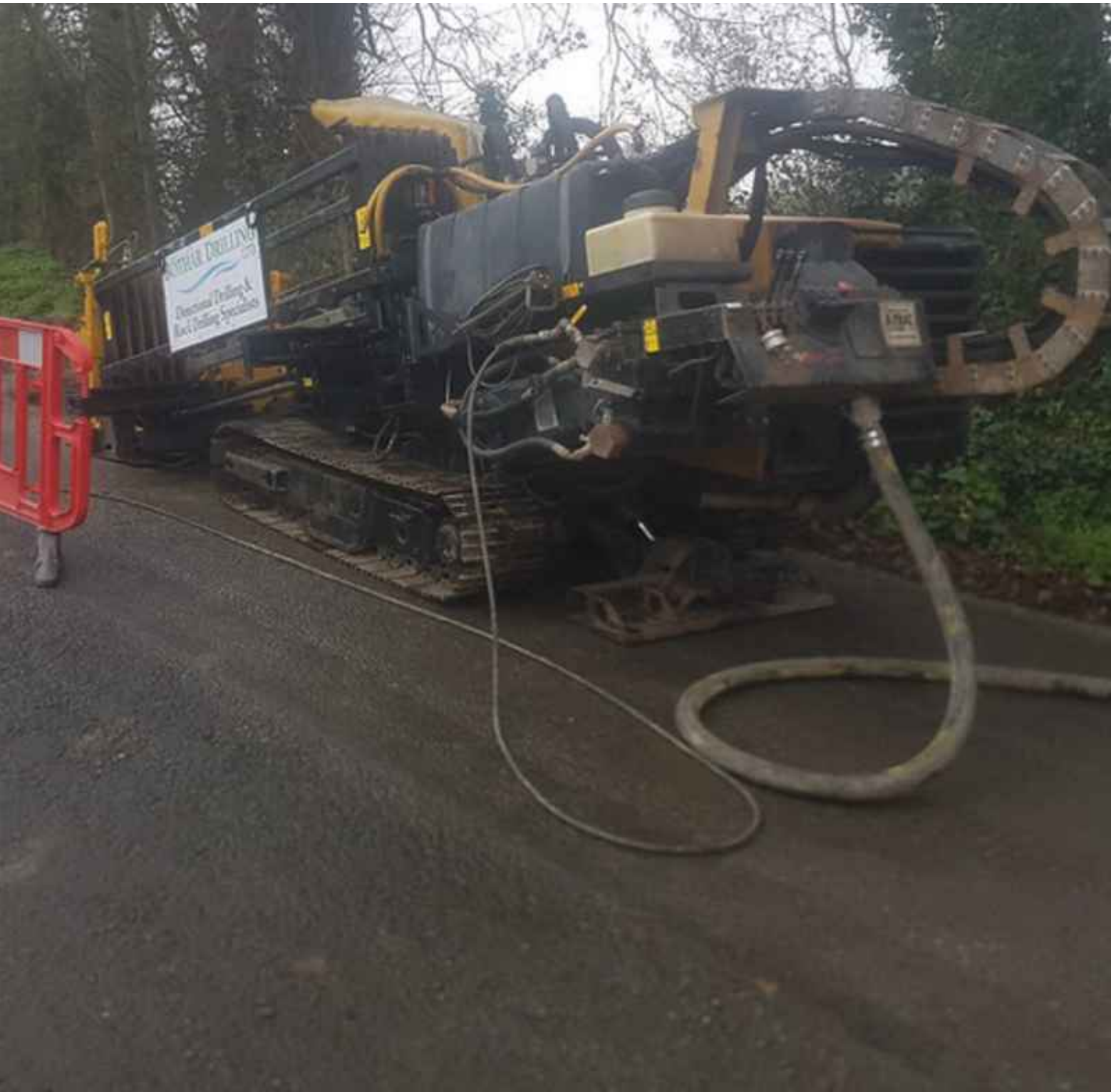
TYPICAL HDD DRILLING RIG
